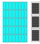
9 96-well delivery plates / 3 source plates Provides maximal capacity for printing arrays in 96-well plates.
